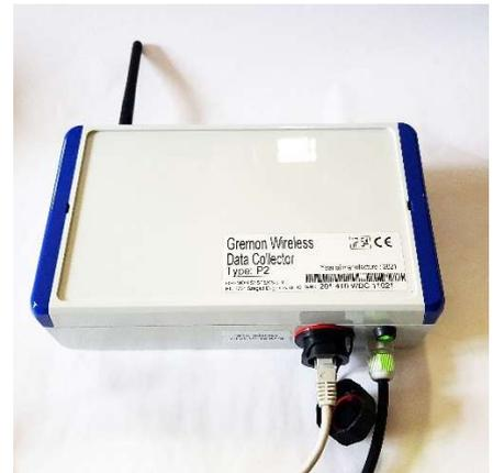
*Data Collector with line power and Ethernet connection. Note the GREEN LED, the network connection is active.*
