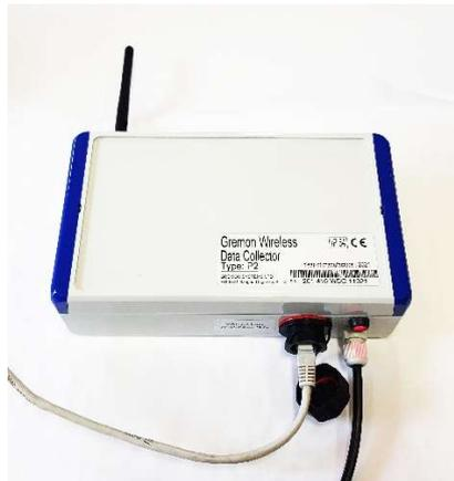
*Data Collector with line power and Ethernet connection. Note the RED LED, there is no active network connection yet.*
